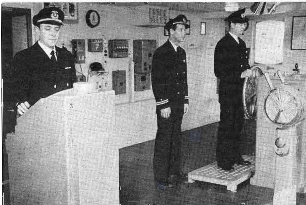
SCENE ON BRIDGE OF THE INDEPENDENCE SHOWING, AT LEFT, THE RCA RADAR UNIT WHICH CAN DETECT OBJECTS WITHIN A 40-MILE RANGE.
