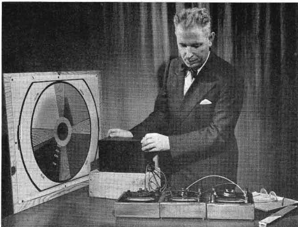
GEORGE C. SZIKLAI, OF RCA LABORATORIES, DEMONSTRATES THE TRISTIMULUS PHOTOMETER, WHICH PERMITS RAPID ANALYSIS OF COLORS.
