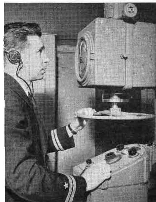
AN OFFICER TAKES THE SHIP'S BEARING WITH THE LATEST MODEL RADIOMARINE DIRECTION FINDER.
